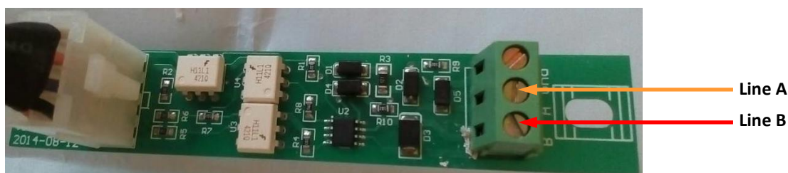
Datian Machines dispenser interface board
