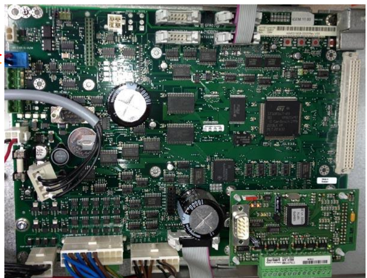
Mepsan dispenser board
